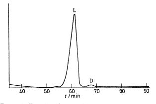
FIGURE 1 Enantiomeric composition of L-leucinol obtained by reduction of L-leucine. Chromatogram of the O-pivaloyl-N-trifluoroacetyl derivative of leucinol on a 2 m  $\times$  4 mm column containing N-lauroyl-L-valyl-t-butylamide coated on Chromosorb P, AW-DMCS
